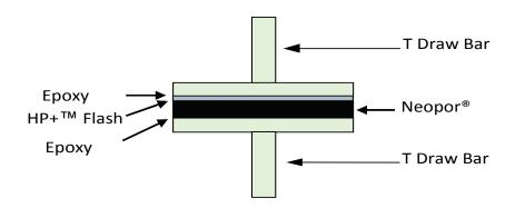
Figure 1. Sample set-up for Adhesion Testing
